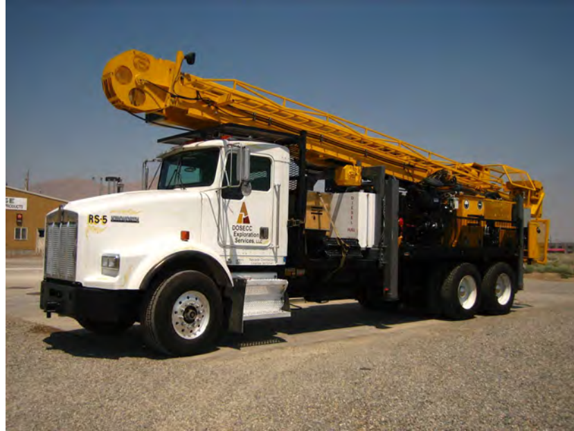
Figure 4. DOSECC's Atlas-Copco 4002 truck mounted drill rig, to used for both deep holes. It has a capacity of 18,000 kg and can lift 2450 m of NQ drill string.
